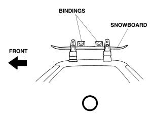
11. If the bindings cannot be positioned between the front and the rear attachments, install the rear binding behind the rear attachment as shown.
