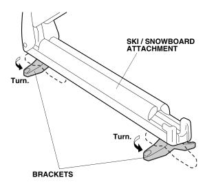
4. Using a wrench, install the ski / snowboard attachment to the front crossbar with four bolts, four collars, and two brackets.
